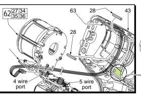
The fuel gauge assembly is a fixed component of the left handle halve (43). Connect the five wire terminal block to the corresponding five wire port on the PCBA.
